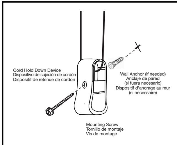
The cord hold down device is used for blinds and shades that have a continuous-loop operating system and a cord.
