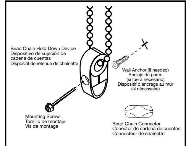
**The bead chain hold down device is used for blinds and shades that have a continuous-loop operating system and metal or plastic bead chains.**
